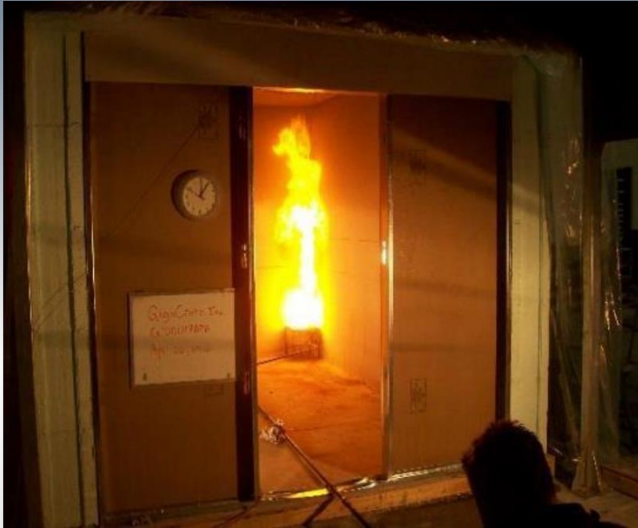
PlasterMax was tested to NFPA 286 a 15 minute Corner Burn Test at 1,400 degrees F as a Gypsum Board replacement over EPS foam.
