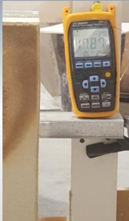
1,797 F registered on thermocouple
