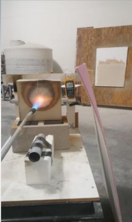
1,700 F flame directly on StuccoMax (E119 does not have direct contact)
