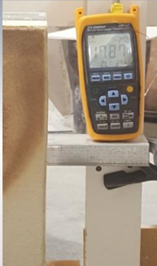
1,797 F registered on thermocouple
